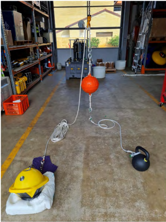
Figure A.1 Mooring build ready for deployment
